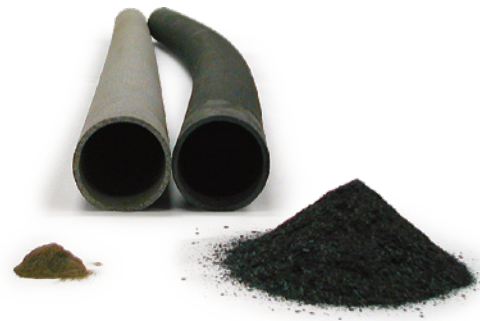
Comparison of Kanthal APMT tube vs. Fe-35Ni-25Cr (after 2300 h at 1100°C [2010°F]). The FeNiCr tube is severely contaminated with oxide flakes.
