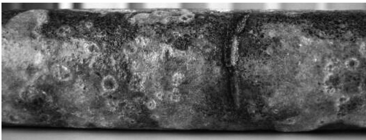
Fig. 3 Conventional SiC element with eroded element surface.
